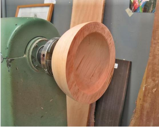
Remove the bowl from the face plate or screw chuck. Place the spigot in the 4 jaw chuck and tighten. The bowl should not bottom out inside the 4 jaw chuck. Turn the inside of the bowl, again practicing tool control. Periodically check that the inside of the bowl is following the outside profile. The inside will start to deviate a little as you get into the bottom of the bowl.
