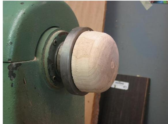
**TIP:** To center a glue block on a dried bowl, turn a 3/8" small spigot on the bottom of the original spigot. Attach your waste block to your face plate or 4 jaw chuck and true up the face. Use a Jacobs chuck in the tail stock, drill a shallow 3/8" hole in the glue block. The glue block will now be centered when you attach it.
