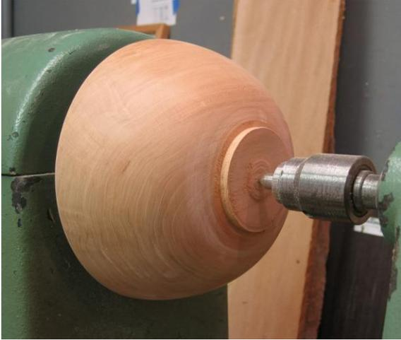
Use a parting tool to part the bowl from the glue block. Reverse the bowl and use the tailstock to hold it against the jam type chuck (from the previous step). Clean up and blend the bottom of the bowl and turn a foot if desired. Sand the bottom.
