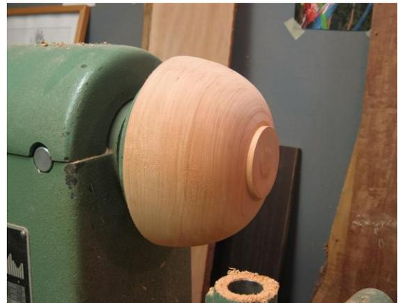
If you're turning dry wood and are going to finish the bowl in one session, glue on a waste block. Hold the waste block in place with the tailstock until the glue dries. True up the glue block. The glue block can either have a spigot turned for a chuck or a face plate can be attached
