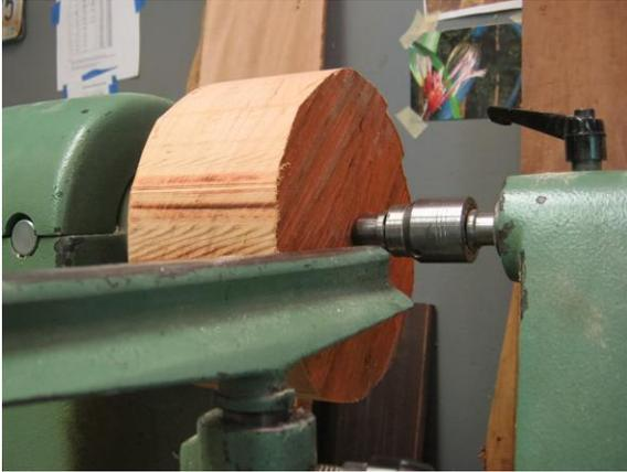
With the blank mounted on the lathe, place the tool rest close to the wood. Rotate the lathe **BY HAND** before turning, checking for clearance between the wood and tool rest.
