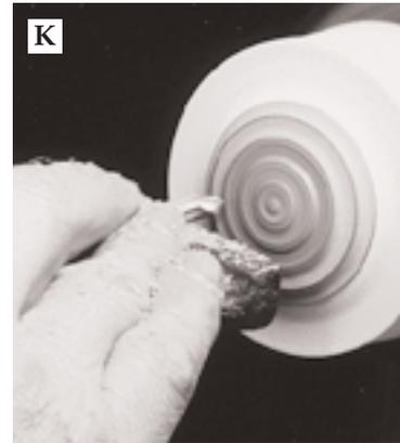
After friction-fitting the lid into a waste block, turn the lid cove lines with a spindle gouge.
