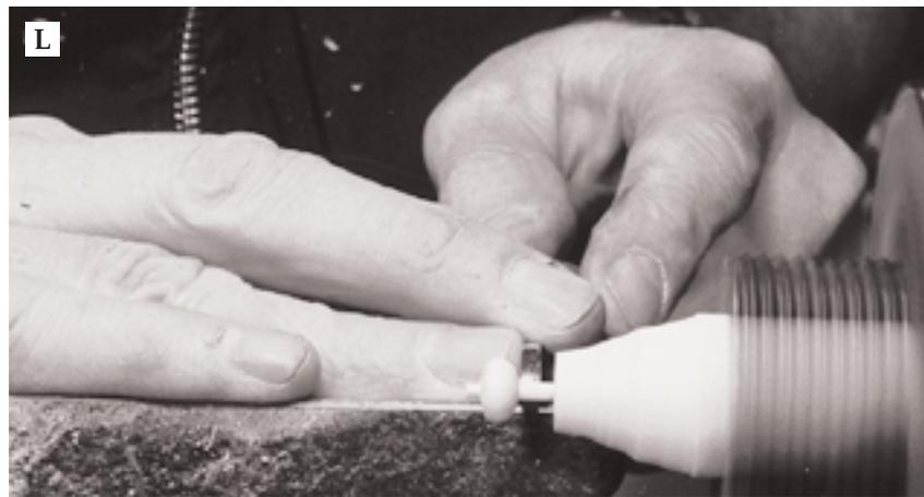
You're nearly done: Turn the knob with a tenon for an "aha!" finishing touch. With the tenon, you'll mount a stick to the knob in the next step (Photo M).
