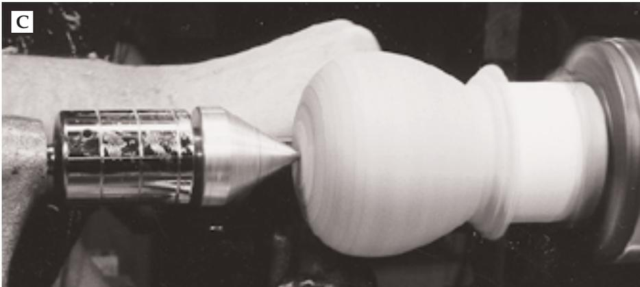
As you rough-turn the body, leave enough material to hollow the interior and texture the surface.
