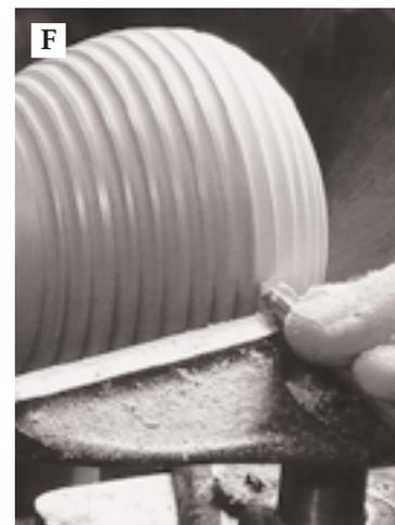
Follow the evenly spaced lines marked on the exterior of the box body to cut the coves with a spindle gouge.
