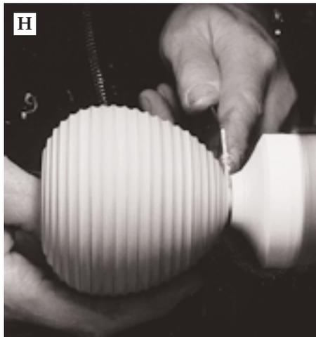
A thin parting tool is ideal to part the box from the waste block.
