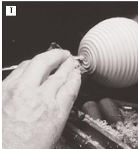
With the body friction-fit into a waste block, turn the coves in the box bottom with a spindle gouge.
