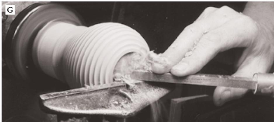
With a round-nosed scraper, hollow the box interior.
