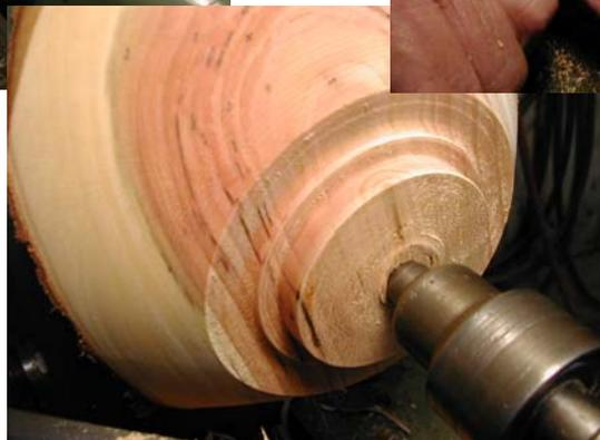
Use a bowl gouge to finish shaping the outside of the bowl. Watch top edge to see shape. Bark can be glued with CA glue if it is coming loose, especially if you will be twice turning the piece. Rough spots can be cleaned up using the shear scrape.
