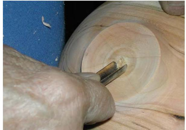
The bowl in this example was turned from green (wet) wood. It does not necessarily need to be as thin as the one pictured below but it is important that it be of uniform thickness and that the pith be cut away from the bottom. Place your finished bowl in a brown paper sack (not plastic) until it is dry. Then you are ready to sand and apply the finish of your choice. If your bowl was turned from dry wood you can sand and finish it right off the lathe
