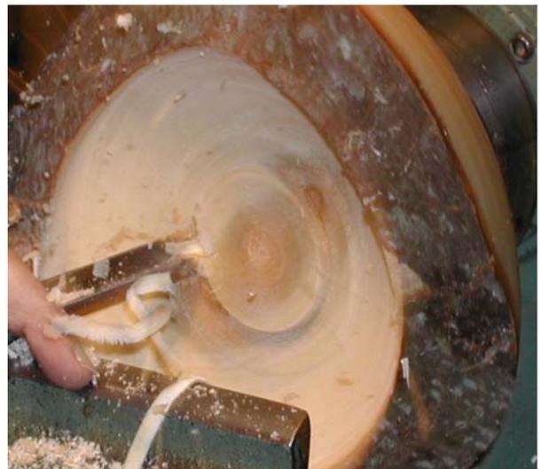
Thin wings to the desired thickness before hollowing the entire center section. This bulk in the interior is needed for support because the wood in the wings begins to flex as it becomes thin.
