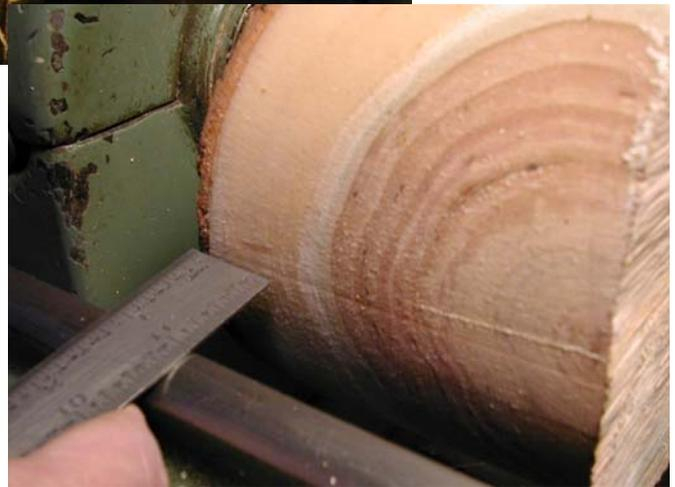
With the tool rest set at an angle, begin to shape the bowl from the bottom up using your bowl gouge. Your first objective should be to remove most of the waste wood on the bottom so you can begin to form the spigot.
