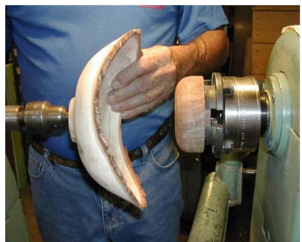
Use a spindle gouge to remove chuck marks and shape bottom as desired. Bring in the bottom by slicing in on lower flute alternating cuts in from the side and then up from the bottom along the axis of the lathe. Make the bottom of your bowl slightly concave so that it will sit level. The thin bottom also makes your bowl less likely to crack.
