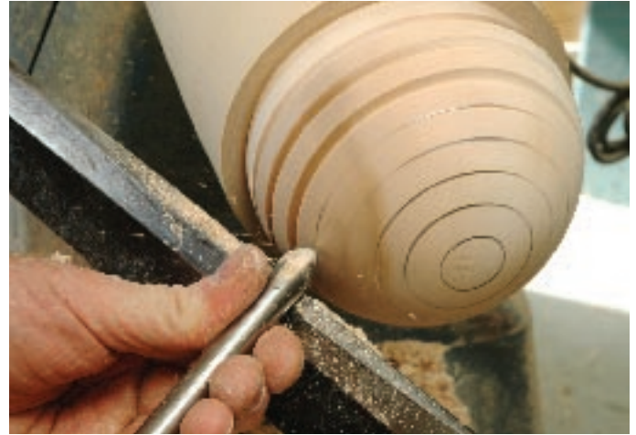
19 With a pencil, draw rings on the bottom of the ball. Carve the grooves with a custom-ground tool as shown opposite below or with a point tool. With a detail gouge, cut the beads and add finishing touches. Then sand to 320-grit smoothness.
