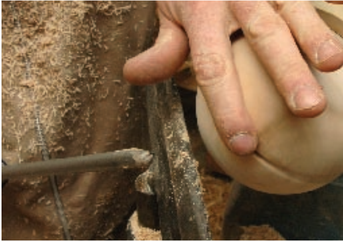
16 Frequently monitor the smoothing process by stopping the lathe and by running your finger over the piece to check for the feel of a false curve.
