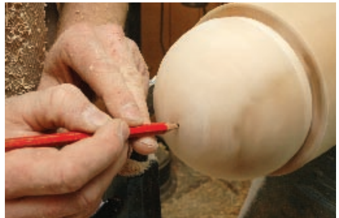
20 Return the ball to the jam chuck—this time with the grooved half facing inward and the assembly joint parallel to the hollow. With the lathe turning, mark the tip of the ball with a pencil. Then, divide the sphere's diameter into eight segments. The drawings below and a compass may help you lay out this step.
