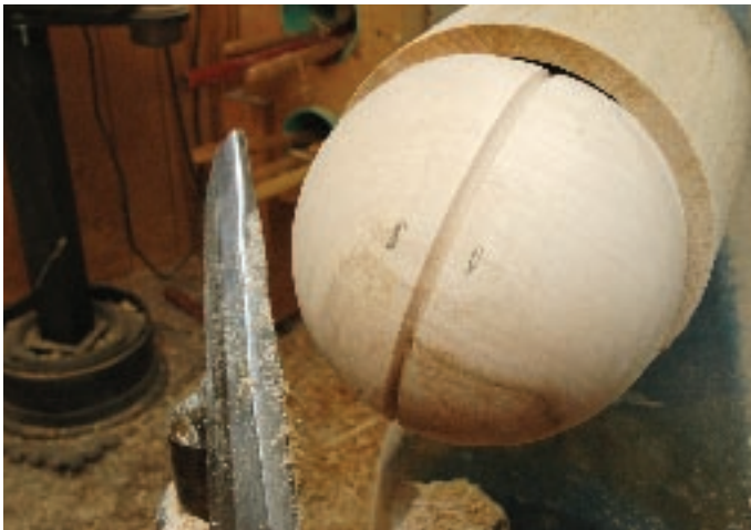
17 Mark two pencil lines approximately 1/4" from the joint. These pencil lines reference what not to remove. At this point, it is important to cease stock removal at the joint. Otherwise, the ball will not end up round. Sand the piece to finish smoothness.
