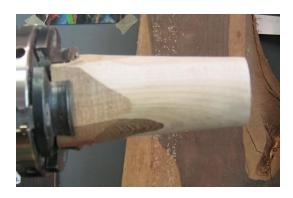
Mount the blank in the four jaw chuck. Then, using your ½" spindle gouge, round the blank down to a cylinder. Be careful that you don't try to round the blank to close to the chuck jaws.
