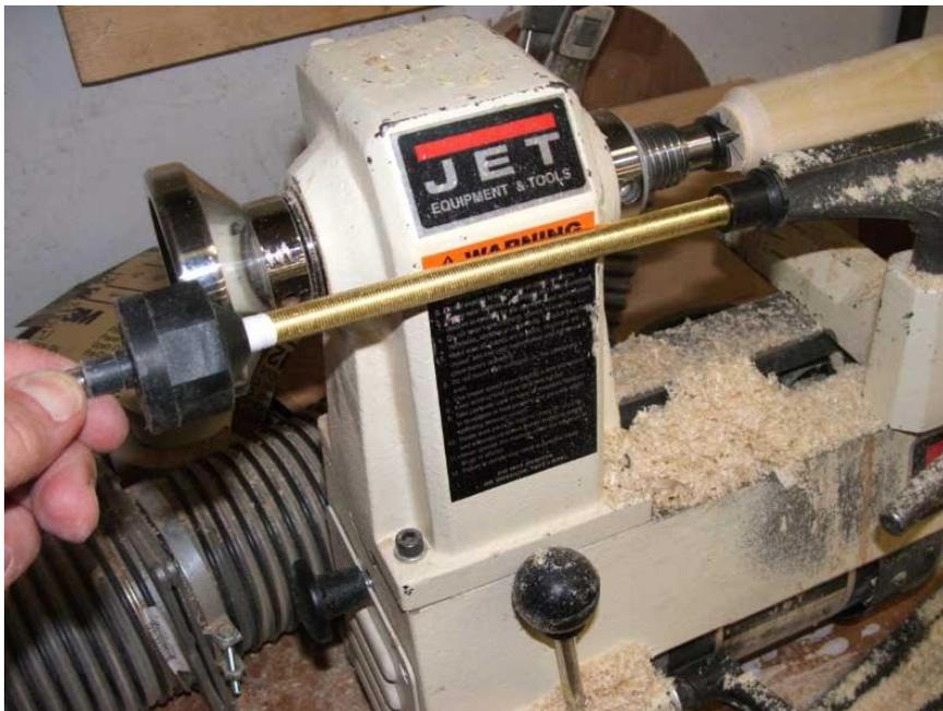
other end is threaded to receive a standard lamp rod. The lamp rod is then inserted through the hollow Spindle and captured by a plastic fitting that has an opening to allow the vacuum into the vacuum chuck head. The fitting snugs the whole assembly just as a draw bar would.
