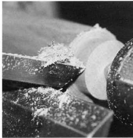
A Scraping Cut
