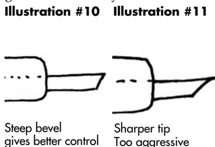
control ... it's just one of those odd cases when the tip is too sharp! As well, when using a deep hollowing scraper with a straight tip, I drop the top surface of the cutter to the centerline of the shaft (Illustration #12) to prevent the tool from grabbing or vibrating on the wood. It's the same principle described above regarding the parting tool. If the
