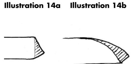
Side view where angles of edges are drawn back to create sharper edges
