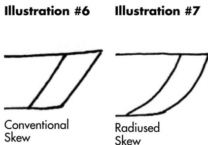
above right, Illustration #7, is that the 'radius' skew presents slightly less physical contact of the edge to the wood during the cut. With less of the edge touching the wood, and assuming the mass and shape of the two tools is the same, the 'radius' design creates a bit less drag on the wood and, therefore, it gives more energy to the cut.
