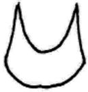
Thin-skew-like edge can cause vibration
