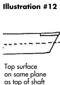
top surface of the tip is above the centerline, or on the same plane as the top surface of the shaft (Illustration 12), watch out!
