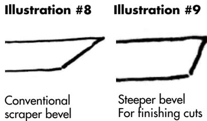
very aggressive on the wood. But it will also wear away quickly leaving a jagged edge that clogs up with dust from the wood and stalls the cut. Conversely, a 120-grit wheel may not raise enough of a burr to do the work. In my experience, a larger burr works well with softer woods and a finer burr works best with harder woods ... but that's only a personal preference, not a rule].
