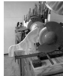
As a last thought, you should also try hand sharpening so as not to become dependent on fixtures. The time will come when the fixture will not work for you or is not available. With the grinder turned off, raise the platform to match the tip angle, and push the tool up the grinder wheel while rotating the tool to keep the side bevel in contact. After practicing a few times you can try it again on an older (and shorter) tool.
