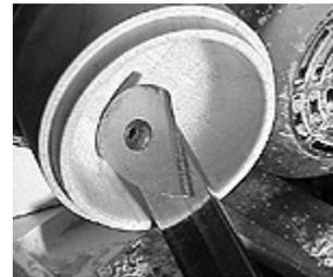
With few exceptions scrapers should be used with the handle raised above center line and the blade trailing below centerline to as to prevent catches – this usually requires raising the tool rest. Rotate the tool rest so that the tool while resting will be slightly skewed over to shear. Holding a scraper on edge is asking for it to be slammed down onto the tool rest with your finger in-between.
