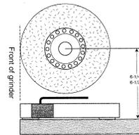
The Verigrind accessory is what holds the gouge and allows for the grinding of the finger nail profile shape. The projection of the tool through the Verigrind should be repeatable (2 inches in average). Tilt the Verigrind forward to the fifth notch in order to set the tip angle. By placing it in the Wolverine V-notch 6.75 inches back from the wheel face one gets good tip and side bevel angles which can constantly repeated.
