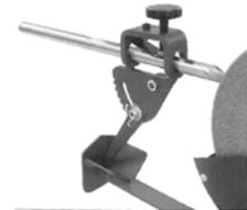
I have made a fixture that resets that distance exactly every time. At the right you can see that fixture and also the small block I use for setting the 2 inch tip projection. Note that the fixture must reference from the *face* of the grinding wheel as its diameter will change over time
